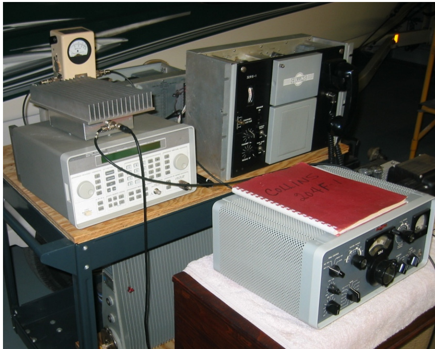
Figure 6. Custom 27 db 120 watt power attenuator constructed for S-Line driver operation. Shown during testing.
